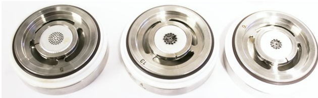
Both ELPI®+ and DLPI+ collect particles in different size fractions on 25 mm filters
