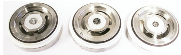
HT-DLPI+ and HT-ELPI®+ collect particles in different size fractions on 25 mm filters
