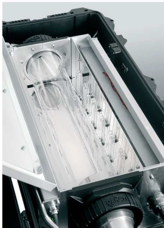
DOFR™ oxidation chamber is made of clear glass and surrounded with 12 UVC lamps operating at 254 nm.
